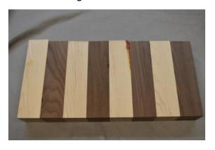
Now it is time to cut the slab into 1 1/8" thick, end grain segments, cut more than you need to accommodate for mistakes and grain matching.
