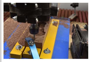
Mount the material to the centerline of the fixture. Secure in the corners with clamps as in the figure above. This is so the clamps do not get hit by the bit during machining.
