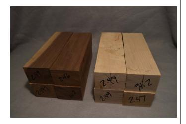
Plane down the material to 1.78"thick. Take care to make this as exact as you can. Cut the material to a width of 2.5 ". Take care to make this as exact as you can. Cut all of the material in to pieces with the length of 8". Now that all of the pieces are machined to size mark the center of the ends and the top.
